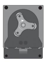
Position the roller at 7h05, turnina it in the direction of the circular arrow.
