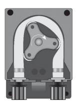
Position the roller at 7h15, turning it in the direction of the circular arrow.
