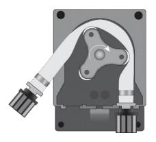
Completely release the connector, holding it taut towards the outside, and turn the roller in the direction of the circular arrow so that the hose is freed up to the right connector.
